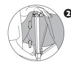
To engage Pull Pin slider at each corner, first lift the fabric off of the slider, then with one hand hold the top of the leg while pushing up on the slider with the other hand. The Pull Pin will engage the hole. Repeat on all 4 corners.
