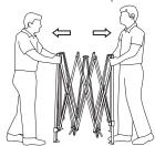
Place your Instant Gazebo frame in the center of area to be shaded. With partner, grasp two outer legs, slightly lift off the ground, and step backwards, stopping at full arms' length.
