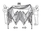
Expand the frame to approx. 2/3 open. Spread the larger fabric (B) over the frame, tuck the fabric under the top vent fabric fingers and using the hook and loop strips, secure the top to the trusses at 8 different points.
