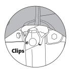
4 Attach the larger fabric to the frame by inserting the 2 clips into the small holes at the top of each leg.
